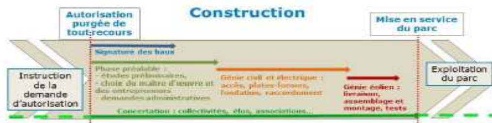
Figure 16 Phasage de la construction
